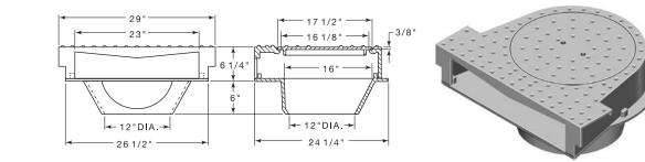
Not recommended for use in areas where large gutter trash objects are prevalent. Curb opening, without gutter grate, allows large trash to enter catch basin and clog lines.
